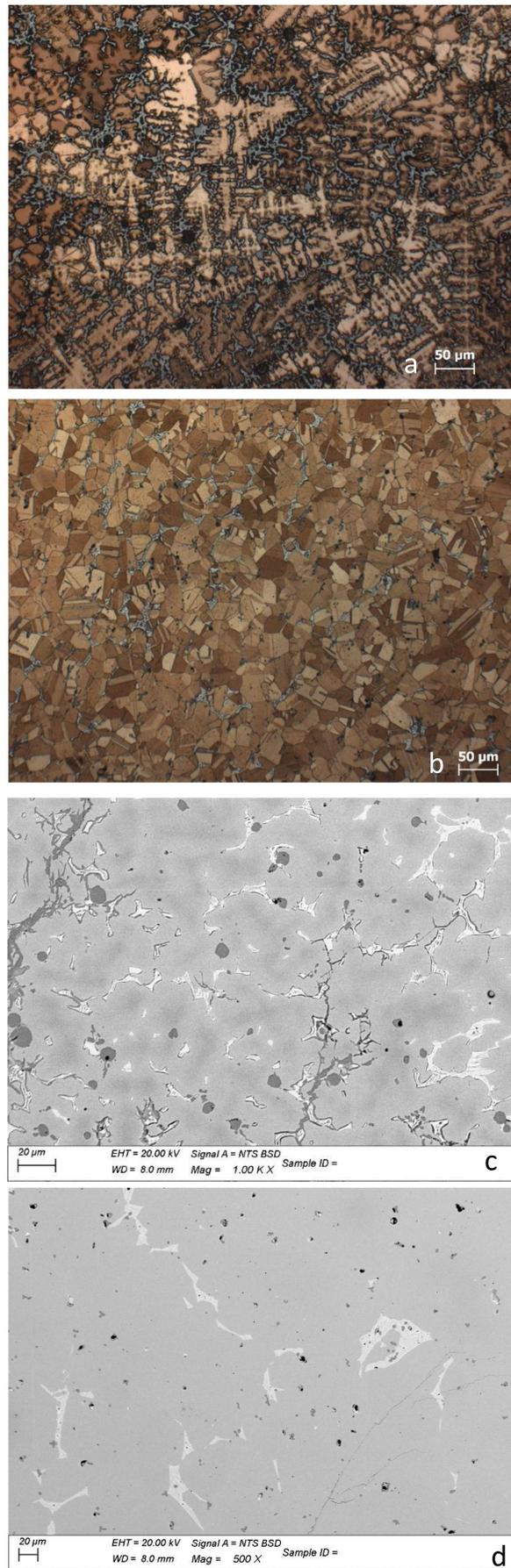
Figure 2) a LOM image for a dendritic structure, b LOM image for a polygonal structure, c SEM-BSD image solidification blank, d SEM-BSD image machined axe
