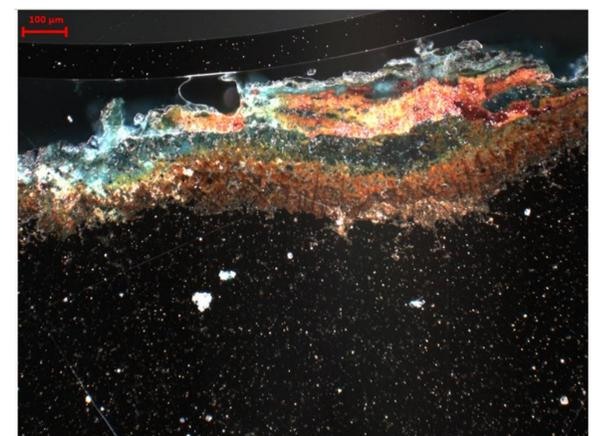
Figure 3) corrosion layer (oxides and carbonates)
